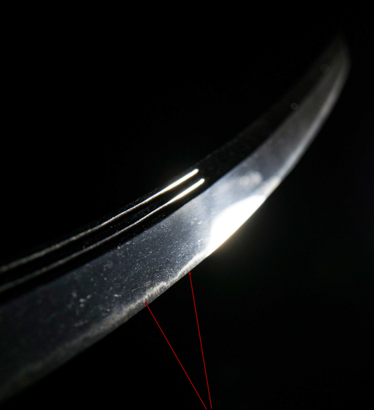
A good view of the tiny nezumi-ashi (rat's legs) that extend from the hamon to the cutting edge, a strong feature of the Naminohira school.
