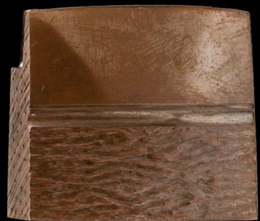
new copper habaki with wood grain file marks
