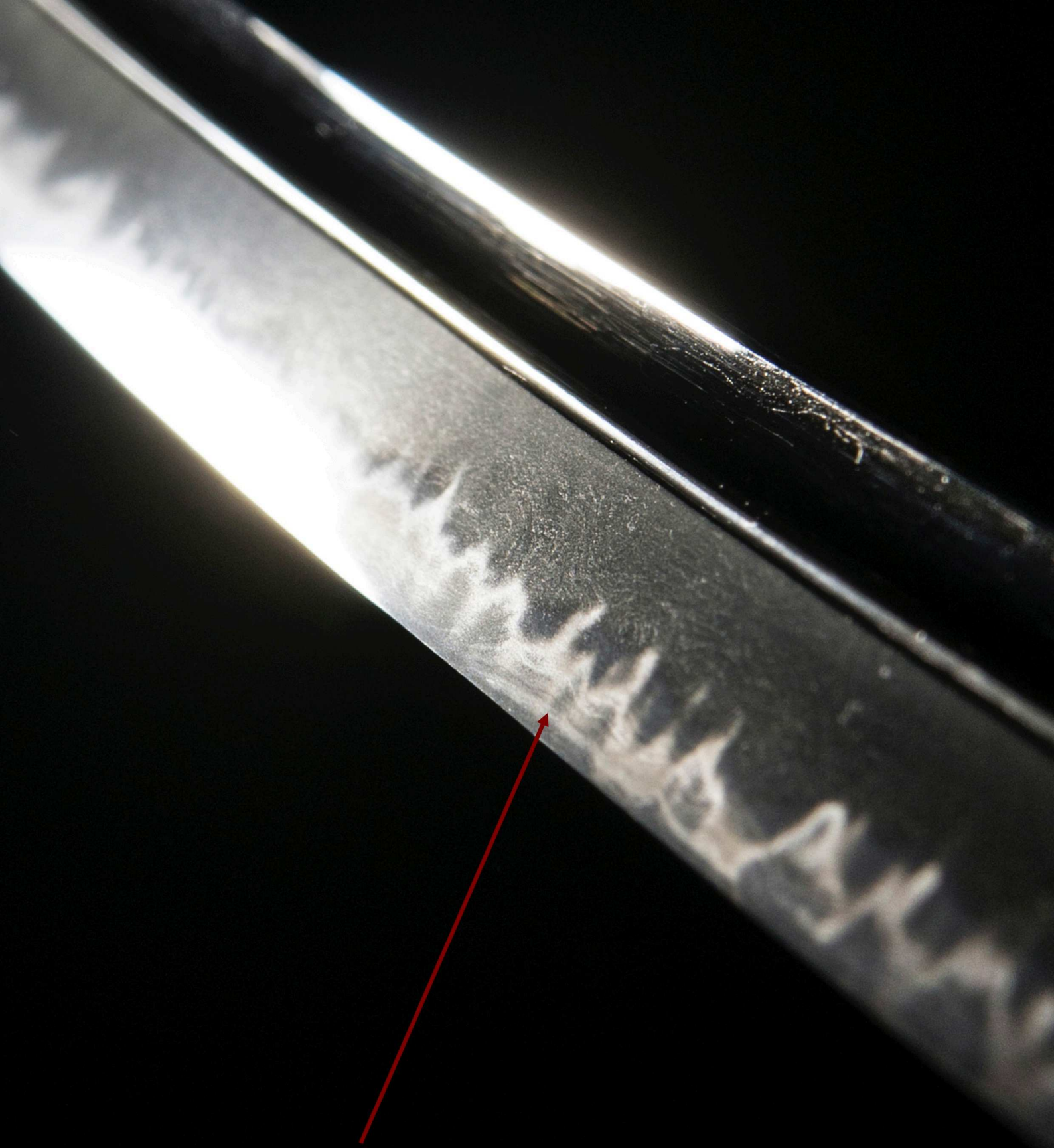
Textbook examples of sunagashi (streams of sand) showcasing a broom line effect inside the hamon.
